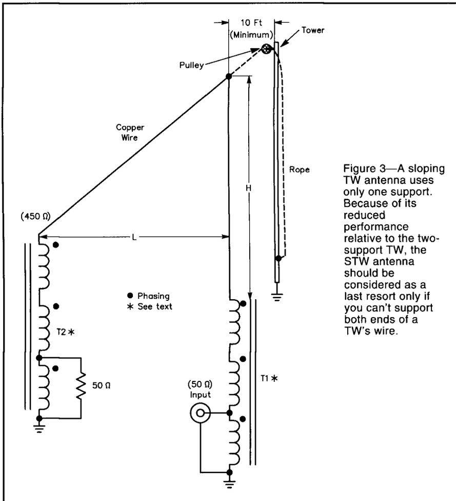
Figure 3—A sloping TW antenna uses only one support. Because of its reduced performance relative to the two-support TW, the STW antenna should be considered as a last resort only if you can't support both ends of a TW's wire.
