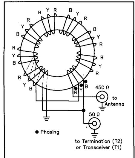
Figure 4—Winding details for the 50:450 Ω impedance transformer.
