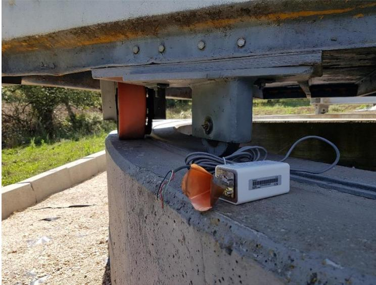
Figure 129 [T6] 22 GHz Horn. (Photo by Michiel Klaassen)
