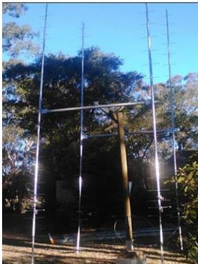
*Figure 102 (O7) Two-by-Two Yagi Antenna Configuration.*
