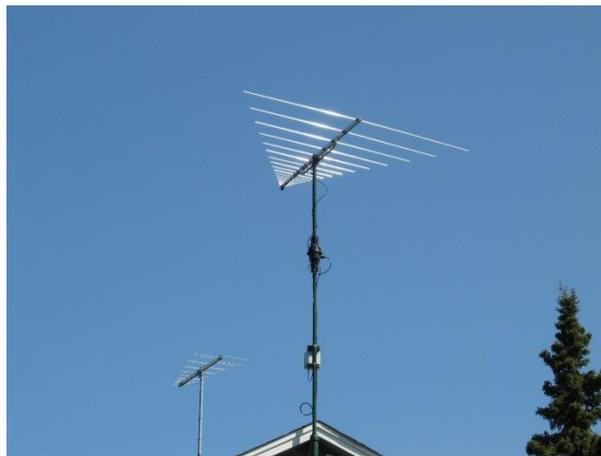
Figure 15: [B2] Gable-mounted, Sun-tracking, 21-element LPDA antenna with design frequency range of 50 to 1300 MHz used in the e-CALLISTO solar radio spectrometer network. (Photo by Whitham Reeve)
