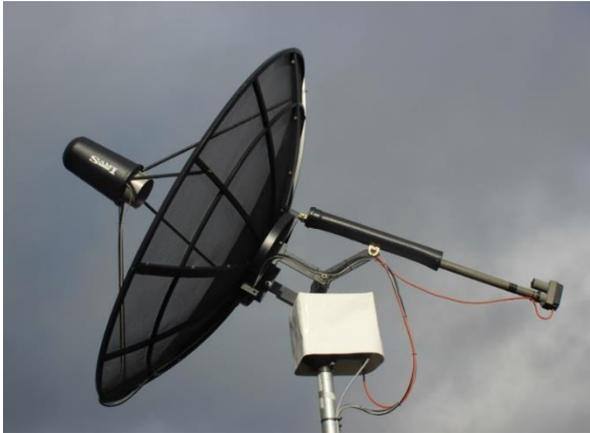
Figure 117: [R1] Figure 1: 2.3-m dish used for the observation.
