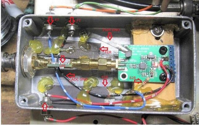
Figure 23:[F4] Detector Box. (Photo by NT4RT)
