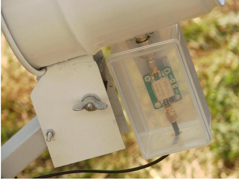
Figure 82(L5) Low-cost wide band amplifier.
