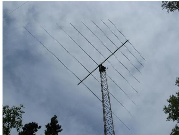
Figure 14: [B1] Tower-mounted, horizontally polarized, rotatable LPDA antenna with 8 elements and design frequency range of 18-32 MHz. (Photo by Whitham Reeve)
