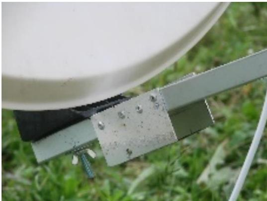
Figure 78 (L1) Saw half trough and fixate with rivets.
