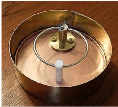
Figure 73: [K2] Original OM6AA Loop Feed scaled to 1420 MHz.
