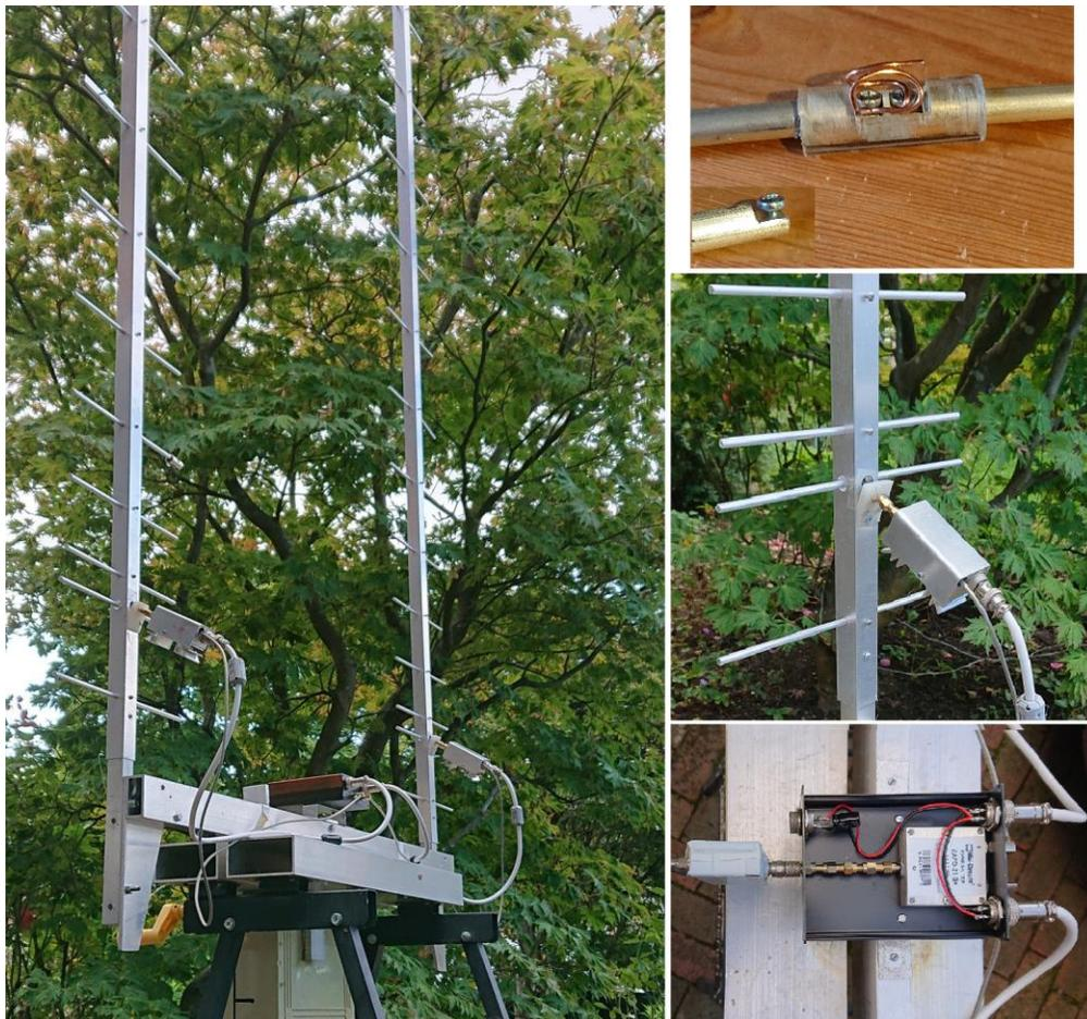
Figure 106: [P2] 2 beam Yagi.
