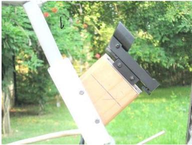
Figure 26:[F7] Telescope Sight. (Photo by NT4RT)
