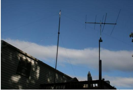
Figure 43:[G4] Installed Antenna on 15 ft mast (height is not critical). (Photo by N2YO)
