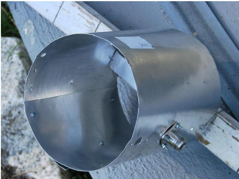
Figure 124 [T1] Feed Connector. (Photo by Michiel Klaassen)
