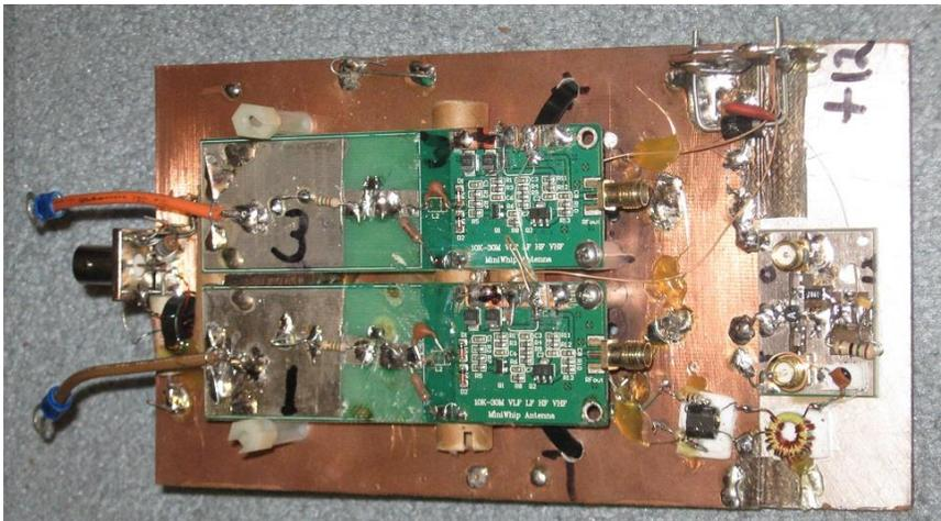
Figure 63: [I16] Complete Antenna Amplifier. (photo by NT4RT)
