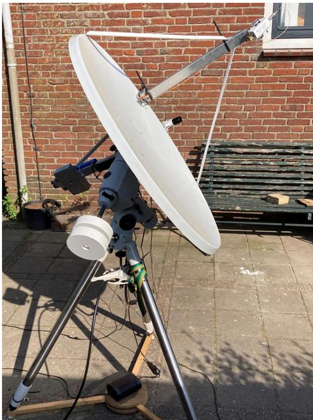
Figure 133: [U1] 1- metre offset dish on HEQ5 mount.
