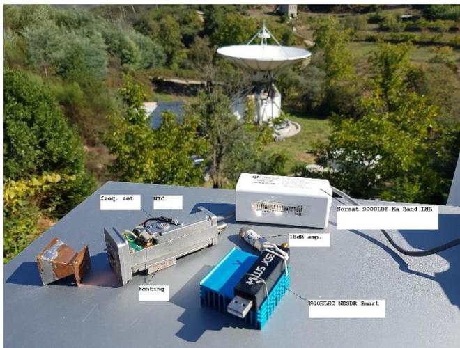
Figure 128 [T5] 22 GHz Setup. (Photo by Michiel Klaassen)
