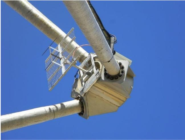
Figure 121: [S2] 408 MHz Feed Antenna photo by WA2JQZ/DSES.
