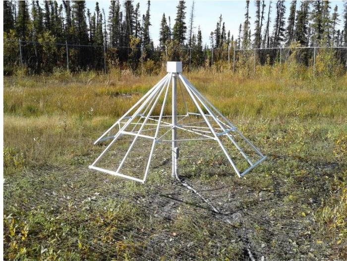
*Figure 16: [B3] Long Wavelength Array (LWA) Antenna is a ground-mounted, crossed-dipole about 1.5 m high. (Photo by Whitham Reeve)*
