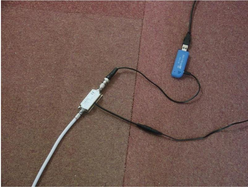
*Figure 80(L3) Inline amp modified as power inserter.*
