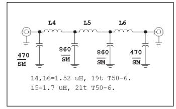
Fig 1.37—Low pass filter for use with the experimental transmitter.
