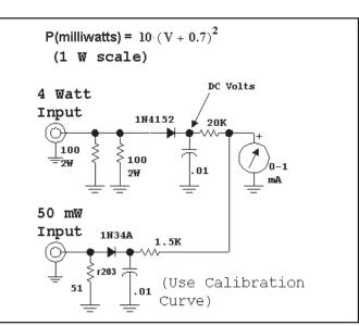
Fig 1.26—Dual range power meter. The 4-W input uses the formula to calculate power in milliwatts. The 50-mW range uses the curve of Fig 1.23.
