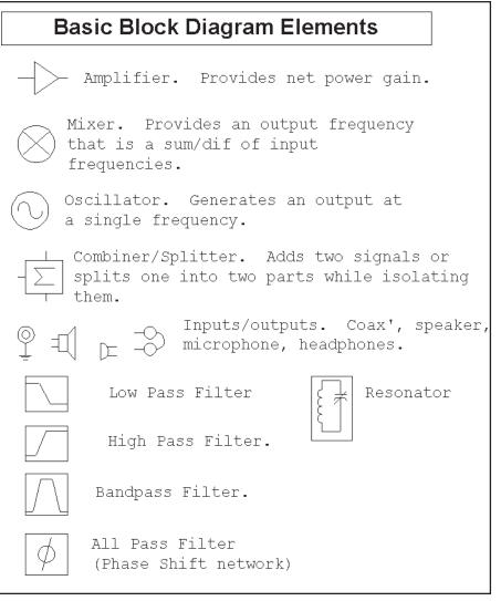
Fig 1.5—Common block diagram elements.
