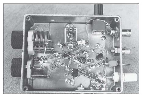
Fig 1.11—Direct conversion receiver assembly.
