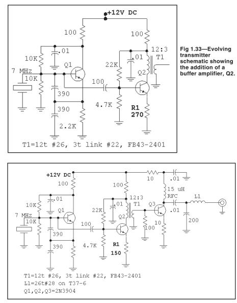
Fig 1.34—A Class C driver amplifier, Q3, is added to the transmitter.
