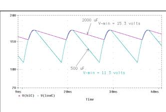
Fig 1.22—Waveforms showing the voltage across filter capacitors of two values when loaded with 0.5 A. See text discussion.
