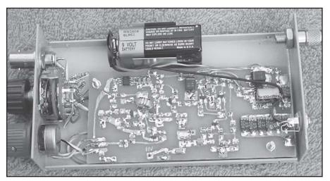
Fig 1.19—Inside view of SMT direct conversion receiver.
