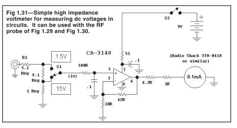
sured without upsetting signals that may be present in the circuit. This circuit can be calibrated with a fresh 1.5-V battery; vary the 6.2-k $\Omega$  resistor if needed.
