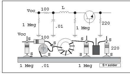
Fig 1.1—A partial circuit illustrating "ugly" construction.
