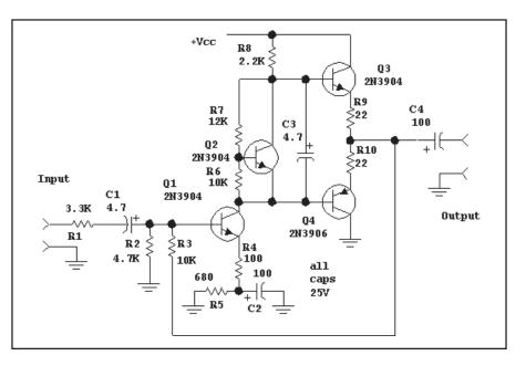
Fig 1.17—Simple audio amplifier using discrete components.
