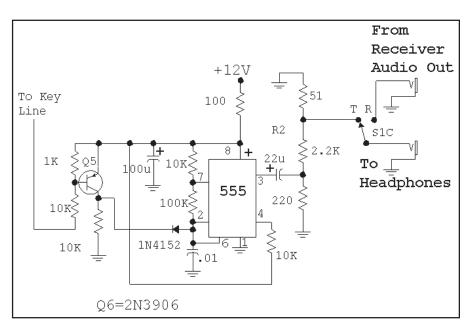
Fig 1.40—Sidetone oscillator for the transmitter. This circuit is also suitable as a code practice oscillator.
