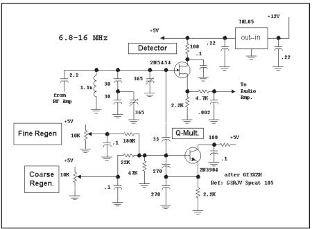
Fig 1.16—Alternative regenerative detector.
