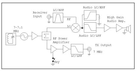
Fig 1.6—Block diagram of a direct conversion transceiver.
