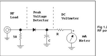
Fig 1.25—A basic RF power meter.
