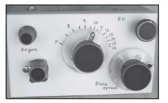
Fig 1.14—Front panel view of the regenerative receiver.
