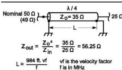
Fig 4—25-Ω to 50-Ω transformer using an electrical λ/4 of 35-Ω cable.
