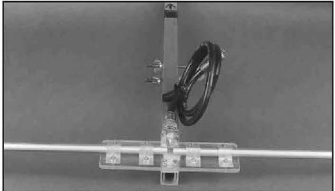
Fig 10(right)—2-turn balun made out of coiled RG-83.
