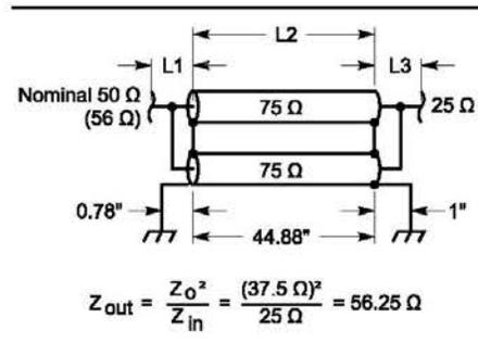
Fig 5—25-Ω to 50-Ω transformer using 75-Ω cable.
