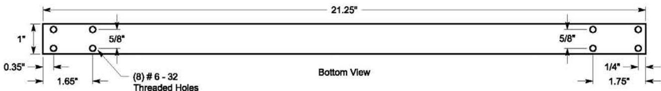
Fig 6—Bottom view of the boom. The top is nearly identical, except that the holes clear #6-32 screws. Use a #36 bit to drill the tapped holes and a #28 bit to drill the holes on top.
