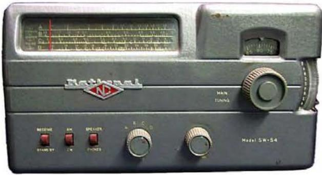
The 1950 SW-54 was one of the few models of ac- and dc-powered receivers made by National. [Photo courtesy of [www.radiopics.com](http://www.radiopics.com)]
