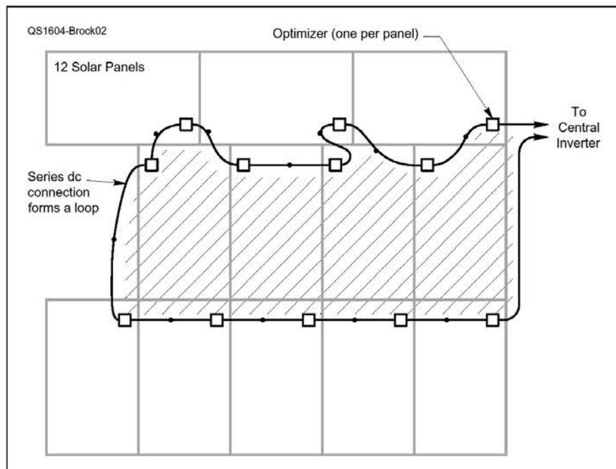
Figure 1 — The standard installation resembles a large current-carrying loop for emitting RFI.
