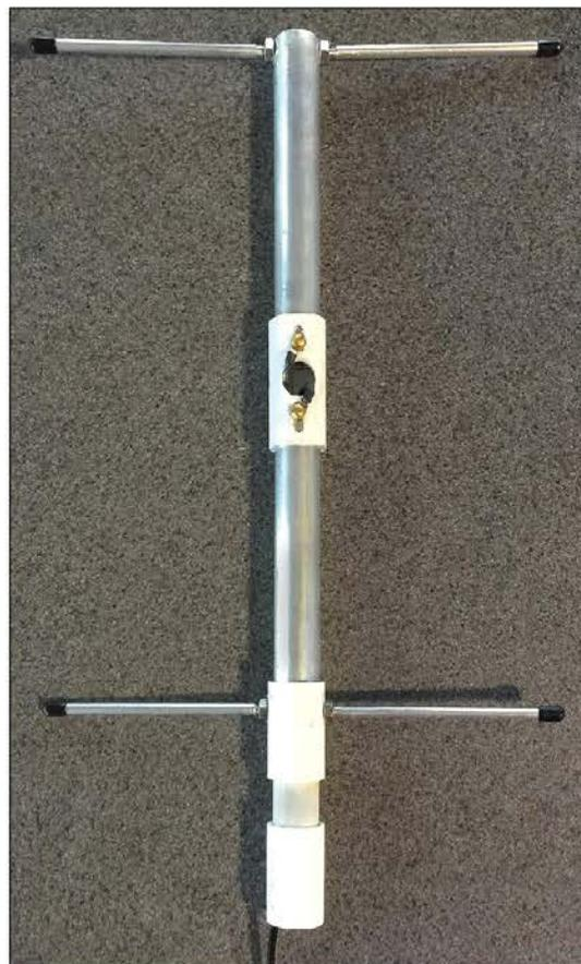
**Figure 5** — Schedule 40 aluminum pipe will fit into PVC fitting to make insulating sections useful in antenna design. Aluminum tubing, however, doesn't fit PVC fittings. [John Portune, W6NBC, photo]
